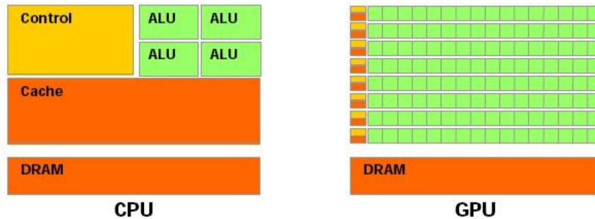
Figure 1-2. The GPU Devotes More Transistors to Data Processing
